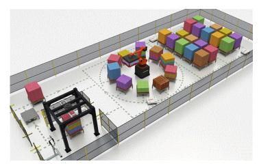
to move between 200-300 layers or stacks per hour. The system provides precise sequencing and high order accuracy, and so can help reduce warehouse labour costs and increase efficiency. You can see a video of <u>CarryStar in operation here</u>, or for further information, go to <u>the Swisslog</u> website here.
